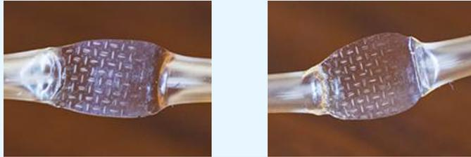
Settings #6 & 7 on a AIE-205 sealer: Sealed, along length of seal, note how the straw flattens to form a large oval, with marks from teflon.
